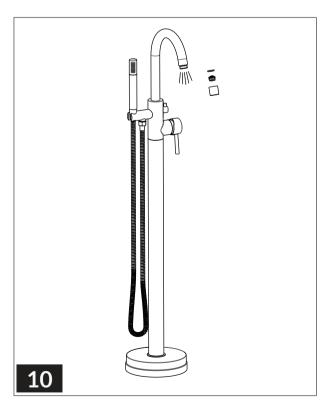
After installation is complete, remove Spray head and rotate handle to the close position. Turn Water Supply Valves on, and check all connections for leak. Flush faucet by running hot and cold water in full position for one minute. Re tighten the Aerator.
