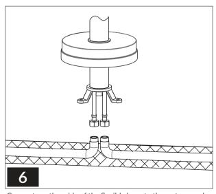
Connect another side of the flexible hose to the water supply pipe. Make sure they are to be fitted into the correct outlets for hot water and cold water.
