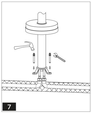
Use the explosion screw to fix the base on the ground. and put the base cover over the base.
