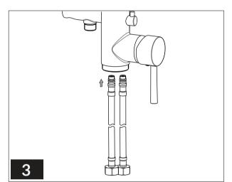
Install the flexible hose now and ensure the flexible hoses are hand tightened into place.(DO NOT USE SPANNER TO TIGHTEN AS IT CAN DAMAGE THE O-RING). The flexible hoses are to be fitted into the correct inlets for hot water and for cold water.
